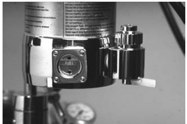
Fig. 17.25. Screw-cap filler system and sight glass for a Fluotec Mark 3 vaporizer. The location of the filler port prevents the operator from filling the vaporizer excessively because liquid will overflow if the maximum level on the sight glass is exceeded significantly. The plastic tubing on the bottom of the filler system facilitates drainage of the vaporizer.
