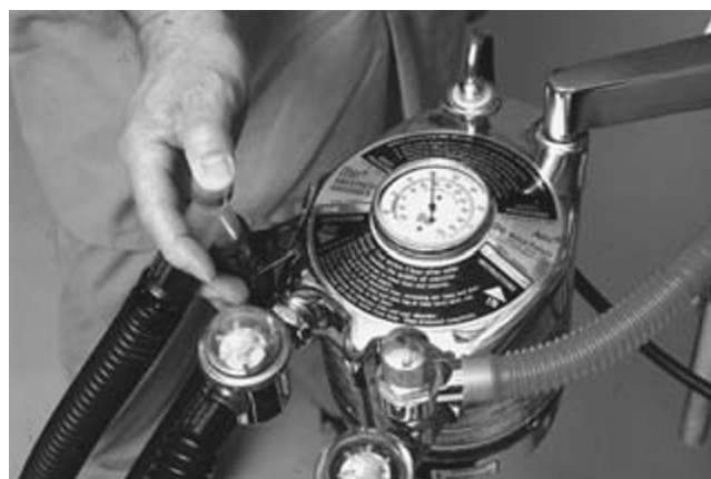
Fig. 17.71. Evaluation of the integrity of a circle breathing system. The pop-off valve is closed, the patient port is occluded, and the system is filled to a pressure of 30 cm H 2 O for at least 10 s, or the leak as determined by use of the oxygen flowmeter should be less than 250 mL/min.
