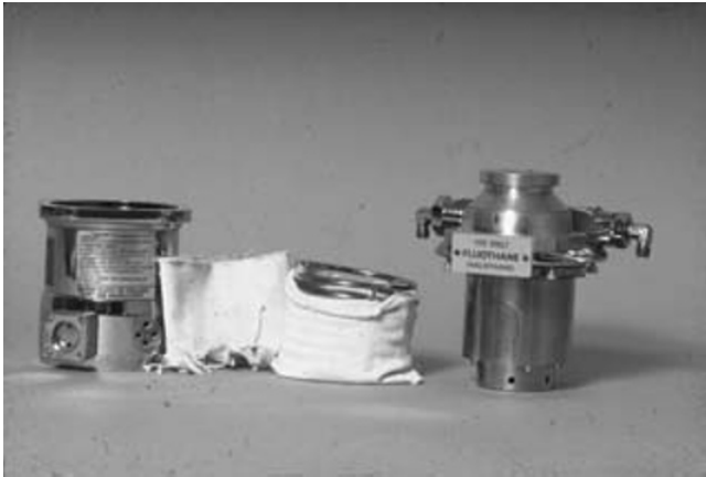
Fig. 17.27. Fluotec Mark 3 vaporizer with cloth wicks. The wicks function to increase the surface area for vaporization of inhalant anesthetic. From Hartsfield. 5
