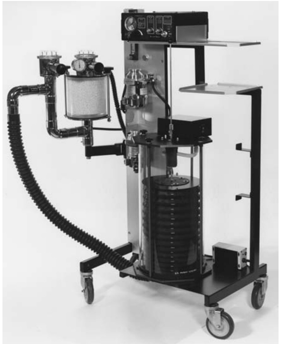
Fig. 18.58. Mallard Medical Rachel Model 2800 Large Animal Anesthesia Ventilator: the ventilator with a Matrx circle system attached ( left side ). The corrugated breathing hose that exits the bellows below the bellows housing is attached to the reservoir-bag port of the circle system. The control console for the ventilator is located at the top of the photograph. The controls for the 2800 are similar to those shown in Fig. 18.48 for the Model 2400V.
