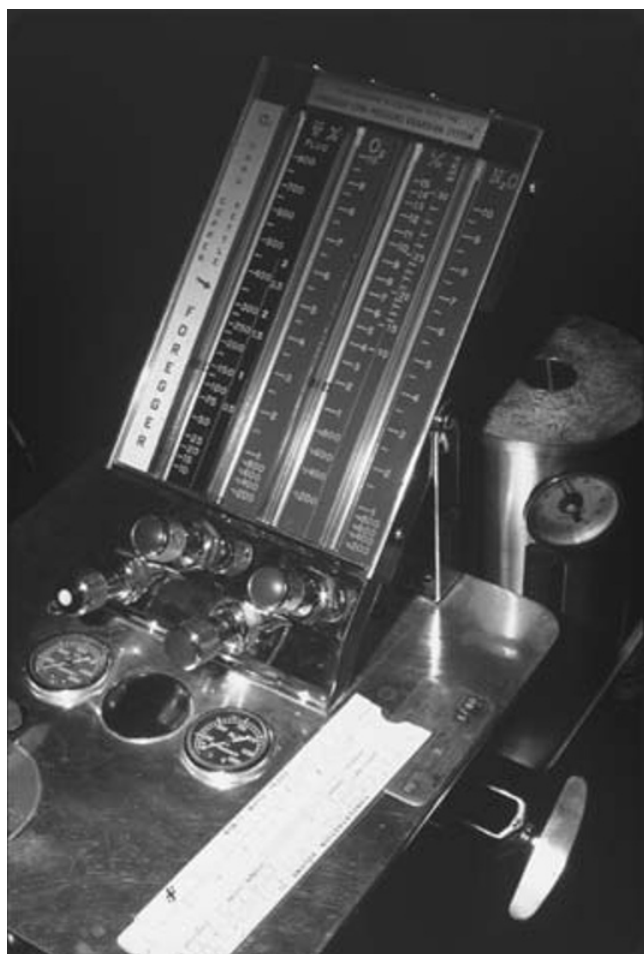
Fig. 17.39. Copper Kettle vaporizer (Foregger, Allentown, PA). The vaporization chamber (copper kettle) with its thermometer is behind the table top ( right rear ), and the vaporizer circuit control valve is attached to the left front corner of the tabletop. The flowmeter cluster from left to right includes the oxygen flowmeter to the vaporization chamber (black scale), two bypass oxygen flowmeters (green), and one nitrous oxide flowmeter (blue). This cluster does not meet recent standards for the arrangement of flowmeters. From Hartsfield. 5
