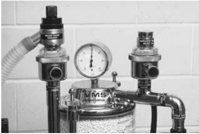
Fig. 17.45. Air-intake valve (negative pressure relief valve) on the dome of the inspiratory one-way valve of a circle system on a Fraser Harlake small animal anesthesia machine. The valve is designed to entrain room air if the supply of fresh gas to the circle breathing system is interrupted. In addition, the pop-off valve is attached to the expiratory one-way valve.
