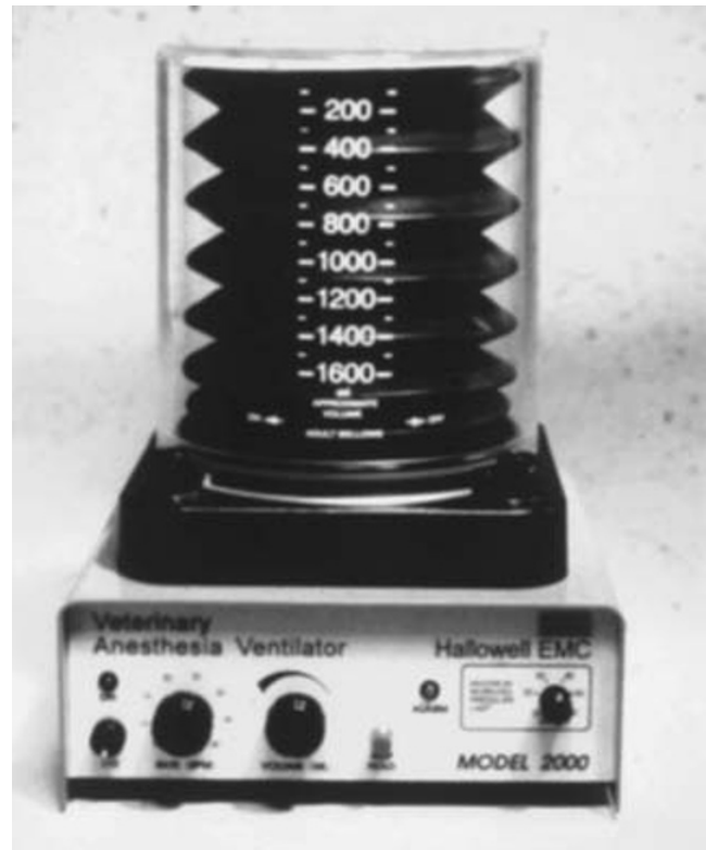
Fig. 18.45. Hallowell EMC Model 2000 Small Animal Veterinary Anesthesia Ventilator (front view). The bellows shown is the medium sized for tidal volumes between 300 and 1600 mL, and the basic control knobs and alarm indicator light are on the front panel. Photograph courtesy of W. Stetson Hallowell.
