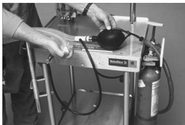
Fig. 17.72. Evaluation of a Bain breathing system (Kendall, Boston, MA) with a complete system check. With all gas flows off, the overflow valve is closed and the patient port is occluded. The bag is filled with the flush valve to a pressure of 30 cm H 2 O, and a leak-free system should maintain this pressure for at least 10 s. If a leak is present, it can be quantified with the oxygen flowmeter and should not exceed 300 mL/min. From Dorsch and Dorsch. 3
