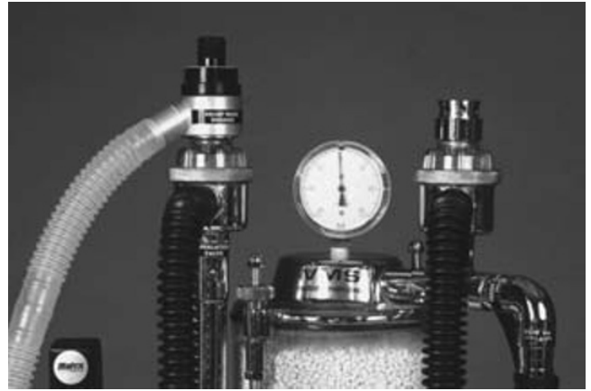
Fig. 17.47. Pop-off valve and manometer on a circle breathing system of a VMS anesthesia machine. The exhaust port (19-mm outer diameter) of the pop-off valve is attached to clear corrugated tubing, which directs waste gases to the scavenging system. The air-intake valve is mounted on the top of the dome for the inspiratory ( right ) one-way valve and functions to entrain room air if the fresh gas supply to the circle system fails.
