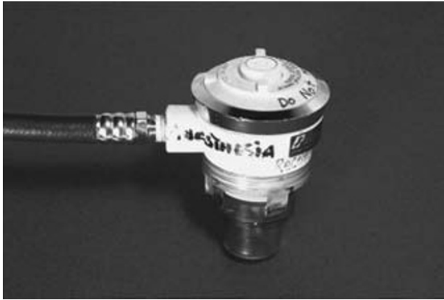
Fig. 18.61. The Elder CPR/Demand Valve. The oxygen inlet is shown with high-pressure oxygen hose connected. The clear plastic connector at the bottom of the photograph will fit endotracheal tube connectors, and the button in the top center of the demand valve activates and controls the flow of oxygen.
