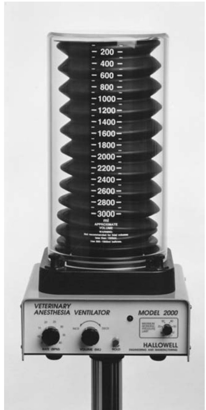
Fig. 18.47. Hallowell EMC Model 2000 Small Animal Veterinary Anesthesia Ventilator (front view). The bellows shown is the largest one for tidal volumes between 0 and 3000 mL. The basic control knobs and alarm indicator light are on the front panel. Photograph courtesy of W. Stetson Hallowell.
