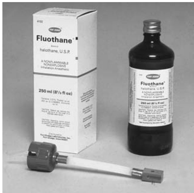
Fig. 17.22. Bottle adapter for halothane vaporizers with keyed filler systems. Such systems reduce the likelihood of introducing an inappropriate anesthetic into an agent-specific vaporizer. The larger end ( left ) of the device attaches to a bottle of halothane, and the opposite end corresponds to the vaporizer filler receptacle. A screw in the receptacle enables a tight seal to be created during the filling process. Bottles of inhalant liquid have a color-coded collar to accept only the correct bottle adapter (see Fig. 17.23).
