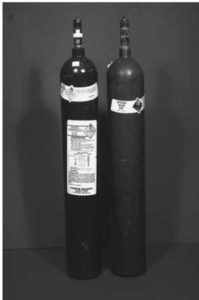
Fig. 17.12. Small (E) cylinders of oxygen and nitrous oxide, with labels and warnings. The diamond-shaped figure on each cylinder's label indicates the hazard class of the contents (yellow for oxygen, an oxidizer; and green for nitrous oxide, a nonflammable gas).
