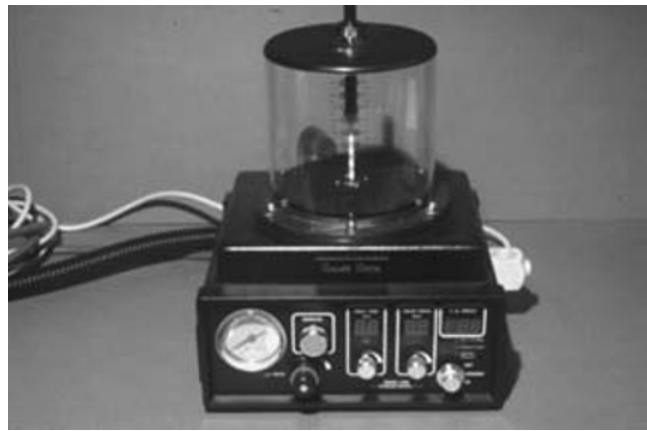
Fig. 18.48. Mallard 2400V Small Animal Anesthesia Ventilator. The bellows is collapsed on the floor of the bellows housing. The tidal volume control is set at approximately 1600 mL. The control knobs on the console are described in the text.
