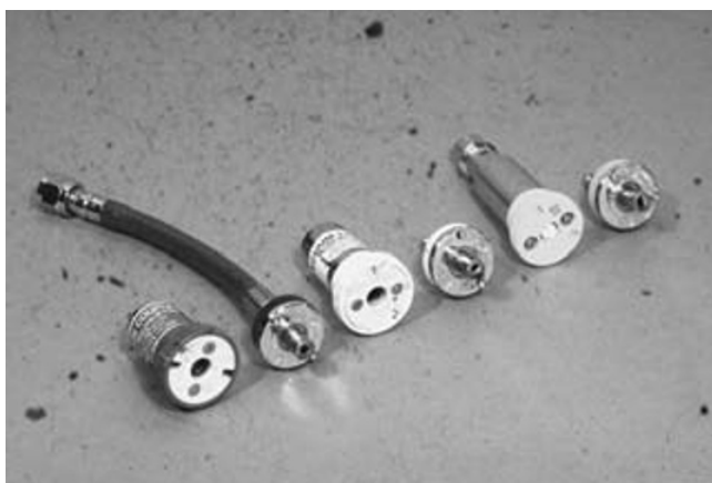
Fig. 17.4. A set of proprietary (Ohio or Ohmeda, Madison, WI) quick connects (quick couplers) for oxygen (male and female on the left ), vacuum (male and female in the center ), and air (male and female on the right ). The female connectors are usually present at the site of use (station outlet) for attachment to the male counterparts from the anesthesia machine or other equipment via high-pressure flexible hose. Inadvertent interchange of the gases is prevented by variations in the spacing of corresponding components of the couplers.
