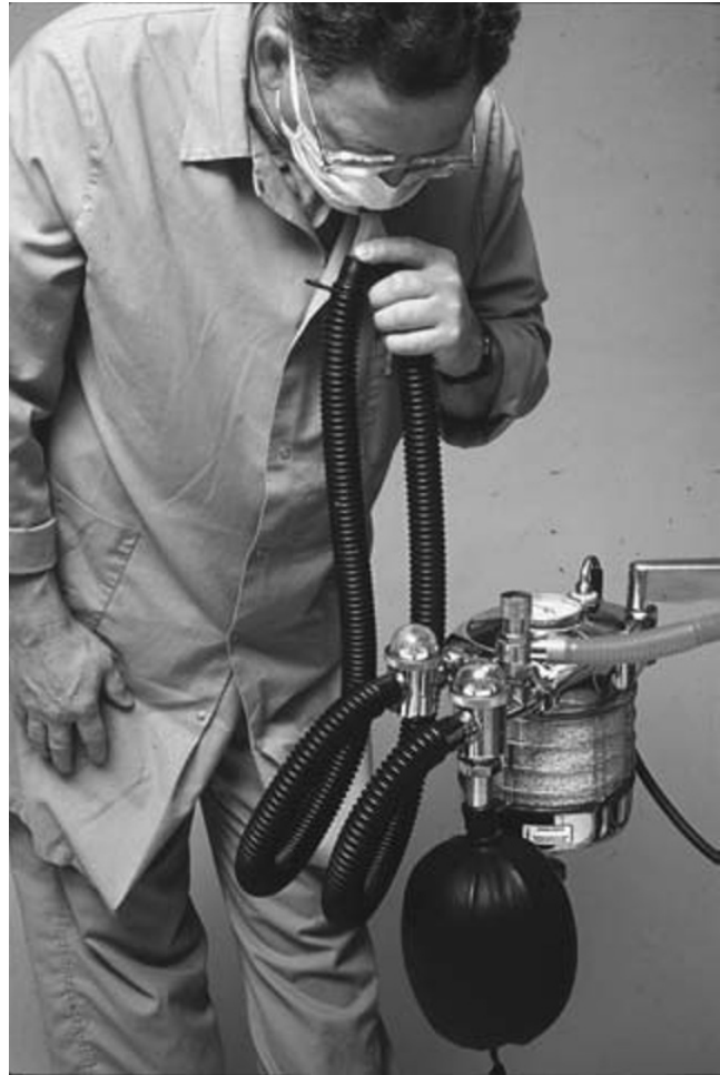
Fig. 17.69. Checking the function of the expiratory one-way valve of a circle system. Wearing a surgical mask, the evaluator exhales through the Y piece and observes the expiratory one-way valve to ensure that the valve disk moves appropriately. The reservoir bag should expand as air moves through the valve.
