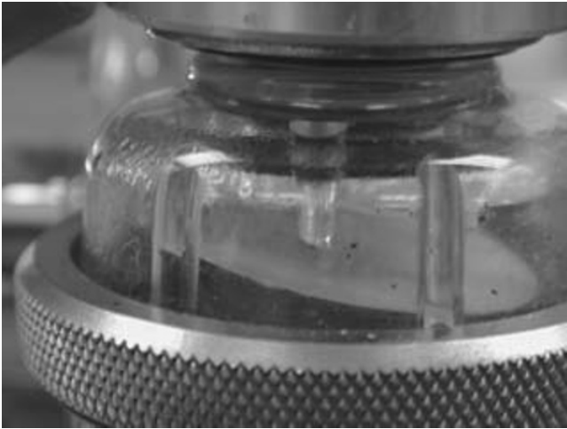
Fig. 53.6. Because of condensation of humidified exhaled gases on the dome and valve, this exhalation check valve has become lodged in the open position, enabling rebreathing of expired gases. An end-tidal carbon dioxide monitor would detect this equipment problem.
