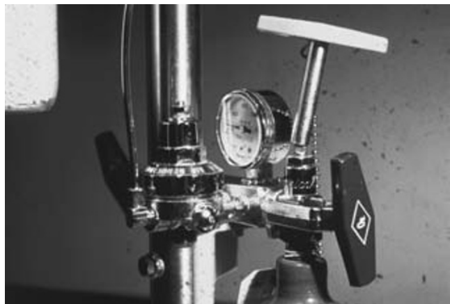
Fig. 17.14. Pressure regulator on a Pitman-Moore 970 veterinary anesthesia machine (Pitman-Moore, Washington Crossing, NJ). The triangular shaped regulator for oxygen is shown in-line between the yoke for the oxygen cylinder and the small-diameter oxygen line to the flowmeter. The pressure gauge indicates the pressure in the cylinder, and the pressure downstream from the regulator is reduced to 50 psi by the regulator.
