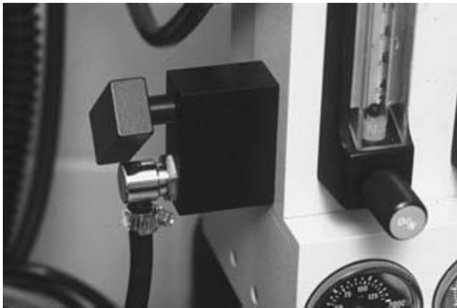
Fig. 17.43. Common gas outlet on a Drager anesthesia machine. The retaining device designed to prevent an accidental disconnection at the common gas outlet is in the open horizontal position.
