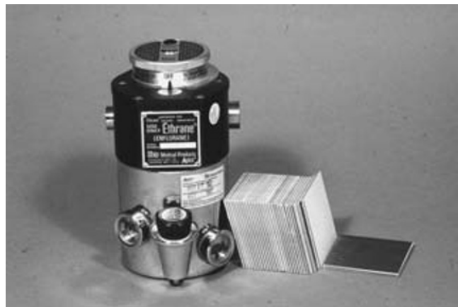
Fig. 17.26. Ohio calibrated vaporizer with paper wicks and copper spacers. The wicks function to increase the surface area for vaporization of inhaled anesthetic.
