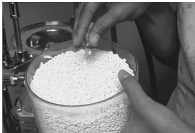
Fig. 17.51. Evaluation of the consistency of soda lime granules. Functional granules are relatively soft and easily crushed, whereas expended granules are hard.
