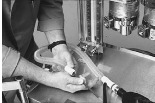
Fig. 17.74. Evaluation of the inner tube of a Bain breathing system. The second step is to occlude the patient end of the inner tube. If the inner tube is intact, the oxygen flowmeter's indicator (e.g., ball or bobbin) should fall (stop flow). From Dorsch and Dorsch. 3
