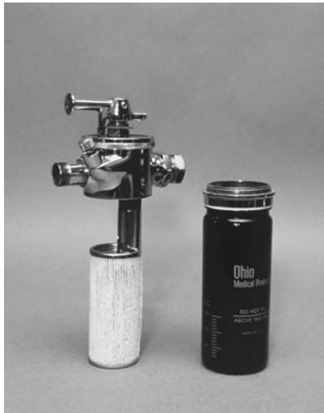
Fig. 17.30. Partially disassembled Ohio #8 glass bottle vaporizer. The cloth wick (left) functions to increase the surface area for vaporization of the anesthetic.
