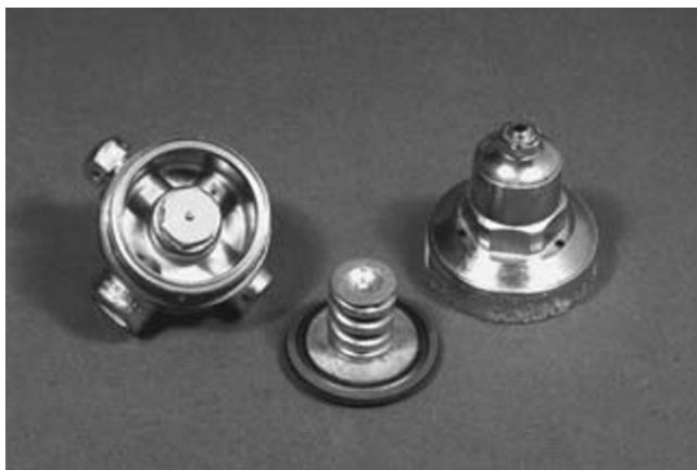
Fig. 17.15. A simple pressure regulator for oxygen that has been separated into its component parts. Shown are the body of the regulator with the entry port for high-pressure gas at 7 o'clock ( left ), the diaphragm and spring ( center ), and the cover ( right ) with holes for pressure relief through the diaphragm and the adjusting screw.
