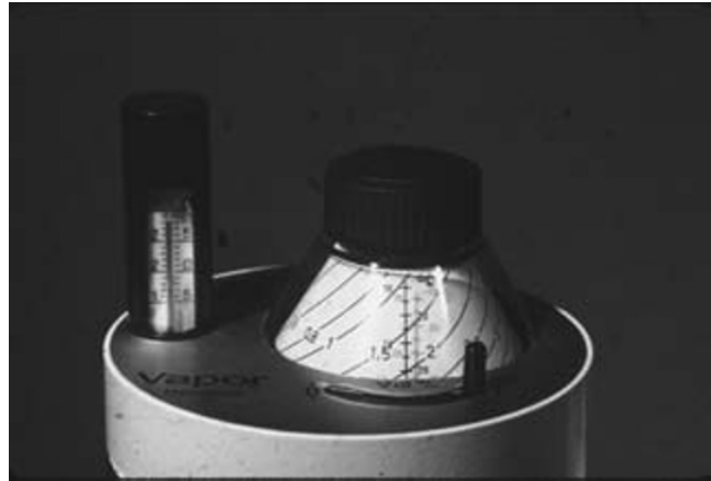
Fig. 17.38. Vapor vaporizer with a control-dial setting of 2% at 28°C. The thermometer ( left ) indicates the temperature within the vaporizer (liquid anesthetic). The control dial is used to manually align the curved line corresponding to the desired anesthetic concentration with the temperature of the liquid anesthetic (the vertical line with hash marks) within the vaporizing chamber. From Hartsfield. 5
