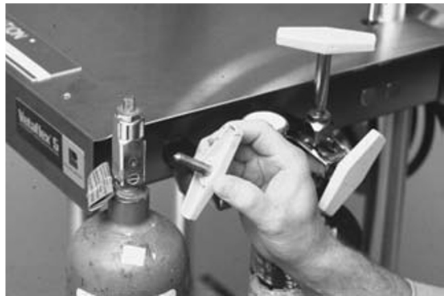
Fig. 17.10. The retaining screw of the yoke and a small (E) cylinder of oxygen next to a Vetaflex 5 veterinary anesthesia machine (Pitman-Moore, Washington Crossing, NJ). The retaining screw has been removed from the yoke to illustrate the pointed shape, which is intended to correspond to the conical depression of the cylinder valve and to secure the cylinder in the yoke. If the cylinder is positioned incorrectly in the yoke and the retaining screw is tightened into the fusible plug (the round, slotted device below the conical depression), the cylinder may decompress rapidly.
