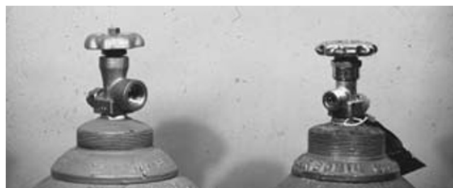
Fig. 17.6. Brass valves on large gas cylinders. The valve outlets on these two cylinders are designed to prevent an inadvertent connection to the wrong cylinder of gases. The valve on the right has external threads, whereas the one on the left has internal threads. The valve outlet for a large cylinder is distinguished by diameter, number of threads per inch, and type of threads (right hand or left hand and internal or external).
