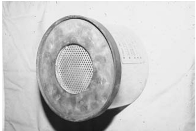
Fig. 17.49. An absorber assembly with an annular ring. The ring diameter, being smaller than the canister diameter, promotes dispersion of gases throughout the canister and helps to prevent preferential flow of gases next to the walls of the canister leading to the development of dead space.
