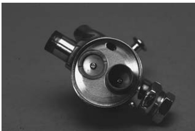
Fig. 17.32. Underside of the head of an Ohio #8 vaporizer showing valves and seats through which gases enter and leave the vaporization chamber. The integrity of these valves in the off position may be lost because of wear or corrosion leading to carrier-gas flow through the vaporization chamber, even when the control lever is in the zero or off position.
