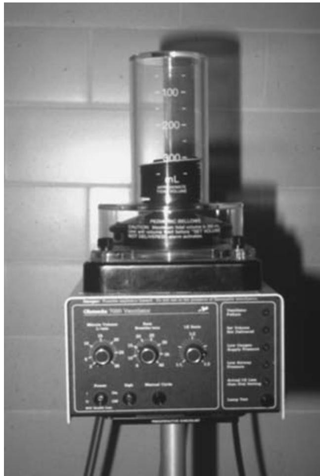
Fig. 18.51. Ohmeda 7000 Ventilator. The control module is shown with six controls on the left two-thirds of the panel and six warning indicators on the right two-thirds of the panel. This ventilator is equipped with a pediatric bellows assembly (0 to 300 mL for tidal volume).
