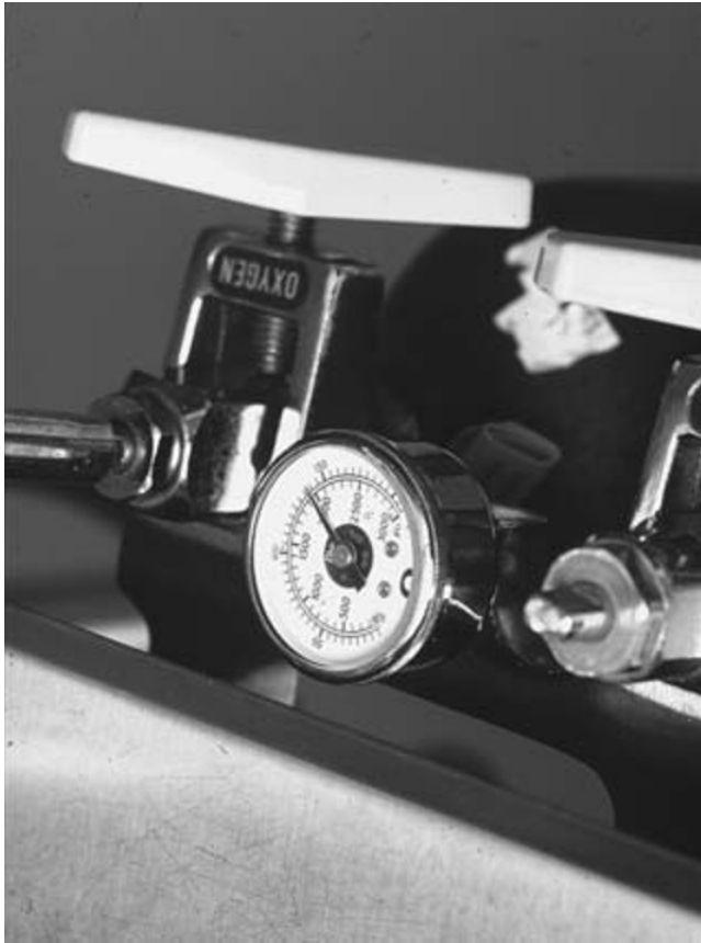
Fig. 17.67. Oxygen cylinder with the pressure gauge reading 2000 psi. An oxygen cylinder should have at least 500 psi before the cylinder and anesthesia machine are used with a patient. With oxygen flowmeters off, the cylinder valve should remain on to allow evaluation of the machine for slow leaks.
