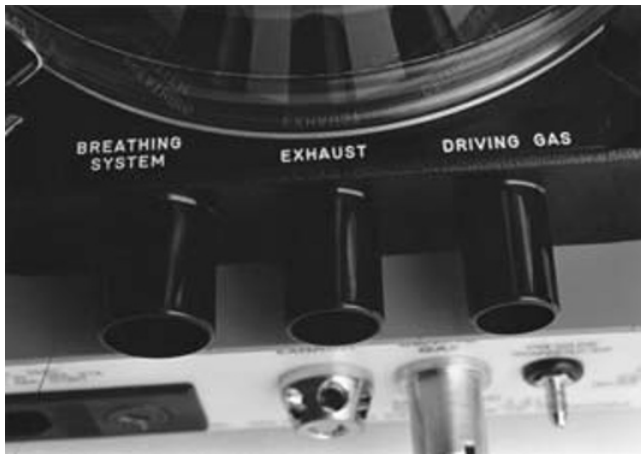
Fig. 18.46. Hallowell EMC Model 2000 Small Animal Veterinary Anesthesia Ventilator (rear view). Note the connectors on the bellows housing for the breathing system, scavenger system (exhaust), and driving gas. Photograph courtesy of W. Stetson Hallowell.
