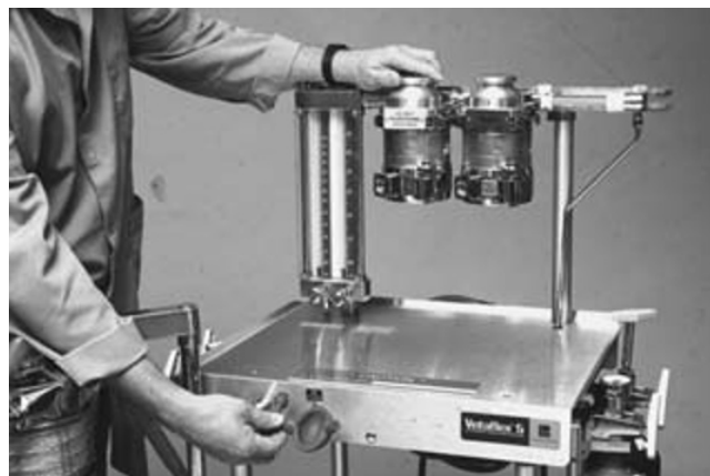
Fig. 17.66. Universal negative-pressure leak test. With all gases off and the vaporizer off, a compressed rubber bulb is attached to the common gas outlet of the anesthesia machine. The bulb should not reinflate in less than 10 s. The test should be repeated with the vaporizer control on. From Andrews. 16
