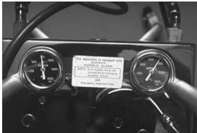
Fig. 17.13. Pressure gauges for oxygen (1900 psi) and nitrous oxide (750 psi) on a veterinary anesthesia machine.
