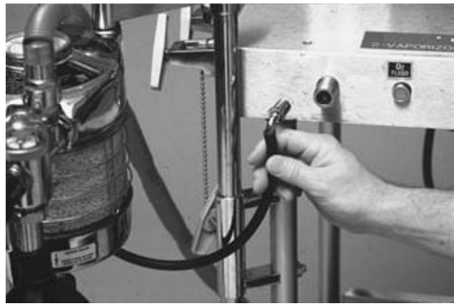
Fig. 17.21. Flush valve and common gas outlet on a veterinary anesthesia machine. The flush valve (labeled on the machine) is protected from inadvertent activation by a circular stainless-steel guard. The common gas outlet (open hole) received a connector to link the anesthesia machine through a rubber hose to the fresh gas inlet of the breathing system.
