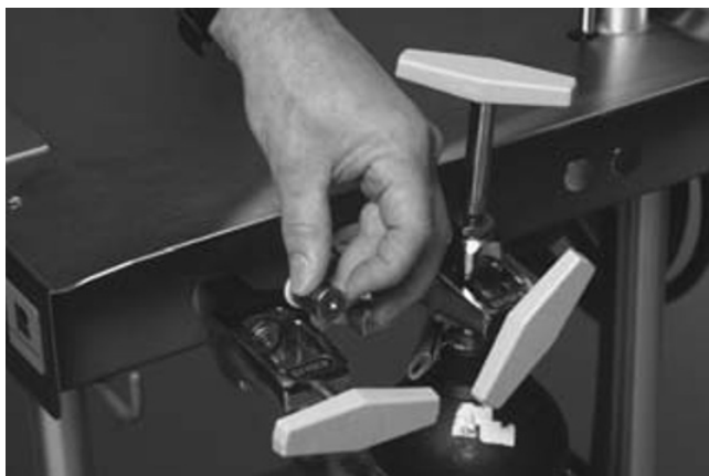
Fig. 17.11. Preparation for inserting a yoke plug into a yoke intended for a small (E) cylinder prior to use of the anesthesia machine. Since only one cylinder is present, the open yoke should be blocked with a yoke plug to prevent gas leaks, even if a check valve is present immediately upstream from the cylinder.
