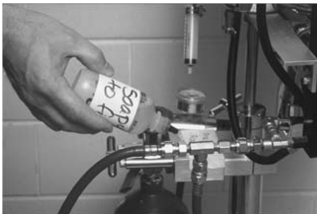
Fig. 17.65. Searching for leaks in the gas piping system of an anesthesia machine. With the cylinder valve on and pressure on the system, soapy water is applied to areas with potential for leaks. Bubbles will form if leaks are present.
