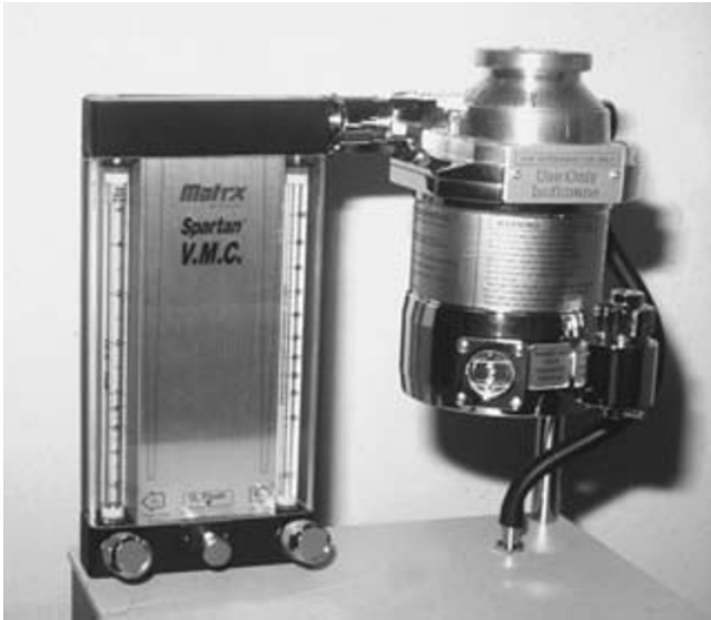
Fig. 17.19. Double oxygen flowmeters on a Matrix Spartan V.M.C. veterinary anesthesia machine (Matrix, Orchard Park, NY). One flowmeter ( left ) is graduated from 0 to 1000 mL/min, whereas the other is graduated from 0.2 to 4.0 L/min. The intent is to increase accuracy at lower flow rates. Two flow-control knobs in parallel offer an opportunity for setting an incorrect flow of oxygen. With two flowmeters in parallel, the total flow is the sum of the flow rates set from each flowmeter.
