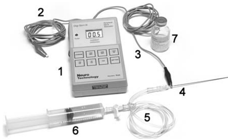
Fig. 20.13. (1) Peripheral nerve-stimulator used as an aid in accurately locating nerves when performing nerve-block procedures: The nerve locator is set at 2 Hz and low output (0.5 mA); the 0.5-mA current delivered to the patient is displayed; (2) the lead wire with red plug (+) and alligator clip for the patient's electrode; (3) the lead wire with black plug (–) and alligator clip for the needle; (4) Stimex insulated needle (22 gauge, 4.25 inches, 0.72 × 10.79 mm); (5) extension set; (6) 20-mL syringe with three-way stopcock, filled with (7) 0.2% ropivacaine hydrochloride.
