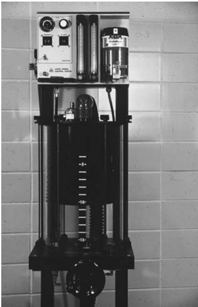
Fig. 18.55. Narkovet-E Electronic Large Animal Control Center: the bellows and bellows housing with markings for tidal volume (4 to 15 L), the corrugated breathing hose from the bellows to the circle system (behind the bellows housing), and the self-locking knob or wheel ( bottom center ) for selection of tidal volume. In addition, the controls for the ventilator and anesthesia machine ( top of the photograph) are included and are shown in detail in Fig. 18.56.
