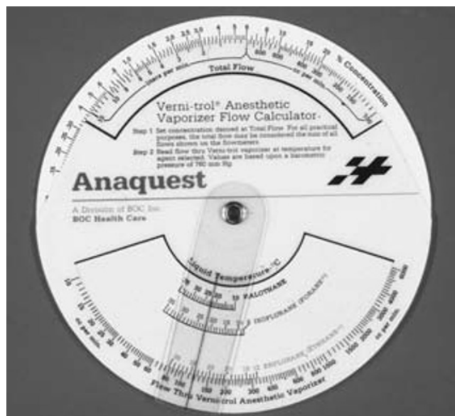
Fig. 17.40. A circular slide rule for calculation of oxygen flow rates for an anesthetic machine with a measured-flow vaporizer. The rule can be used for several different anesthetics at various total flow rates over a range of temperatures. This circular slide rule shows that 120 mL of oxygen must be supplied to the vaporizer to produce 3% halothane at a total gas flow rate of 2 L/min at a vaporizer temperature of 23°C.
