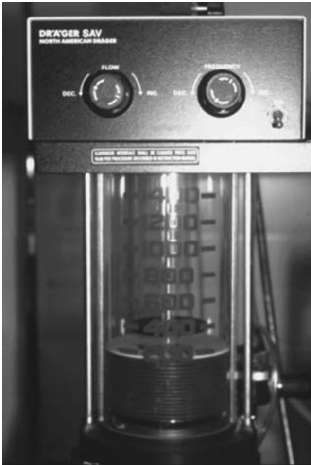
Fig. 18.44. Dräger SAV (small animal ventilator; front view). The ascending bellows and the bellows housing with the tidal volume marked in milliliters are shown in the bottom of the photograph, and the inspiratory-flow control knob ( left ), the frequency control knob ( center right ), and the power switch ( far right ) are shown in the top of the photograph.
