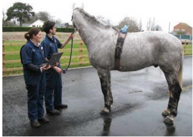
FIGURE 1-7 Televet electrocardiography (ECG) system (Kruuse, UK) being used on a horse, Philip Leverhulme Equine Hospital, University of Liverpool.
