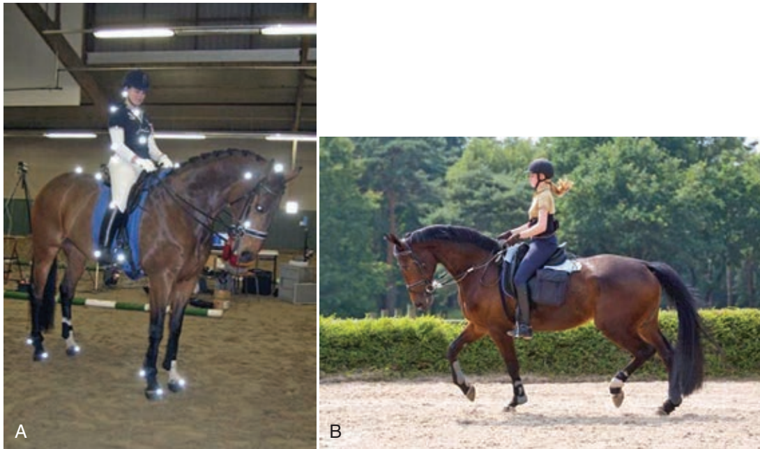
FIGURE 18-1 Two horse-rider combinations with instrumented tack. A , Horse-rider combination with normal force sensors incorporated in a blanket underneath the saddle and between the legs of the rider and the horse. On both rider and horse infrared light reflecting markers are placed to measure kinematics. B , Horse-rider combination with strain gauges incorporated between bit and reins and a saddle force device underneath the saddle. (Courtesy of Bit Horse Magazine, Lonneke Ruesink.)
